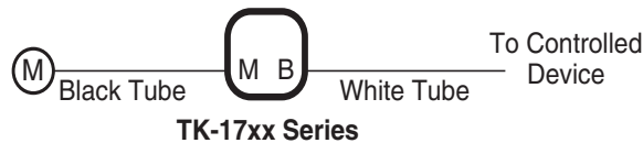
TK-17xx Series Figure 4 Typical Application.
